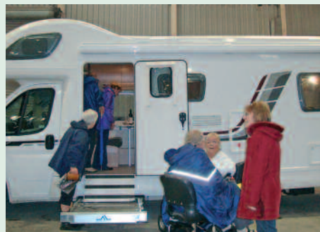
External view of John's motorhome showing entrance lift
